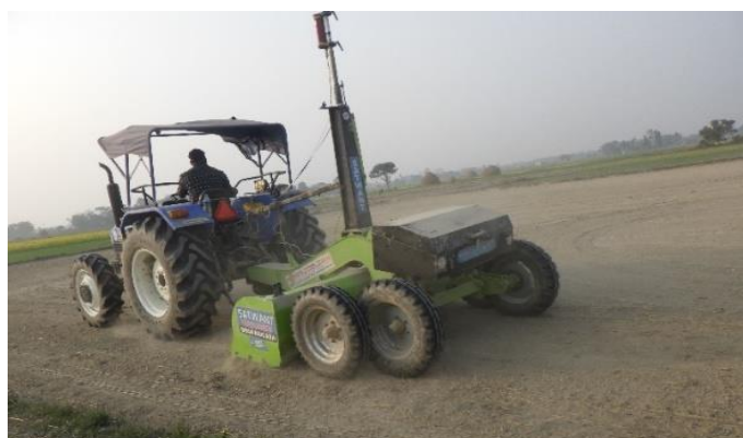
Land Levelling demonstration using Laser Land Leveller in farmer’s field conducted
